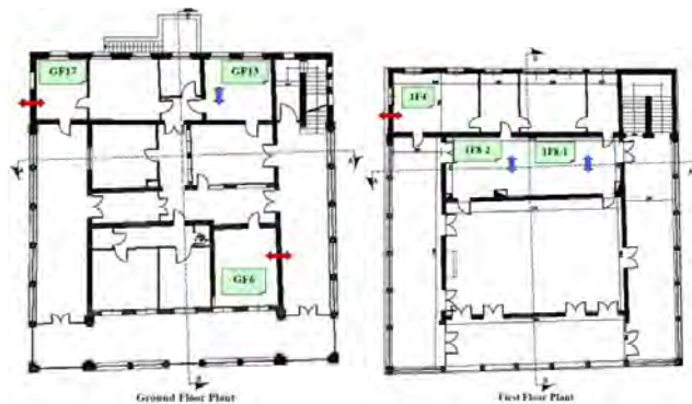
Figure 52_Plan view of the ground and first floor, with the position of U-value measurements
