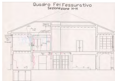
Figure 48_ Crack pattern survey on a vertical section
