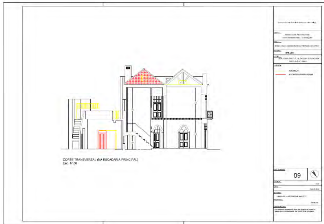
Figure 4_ cross section in the main staircase
