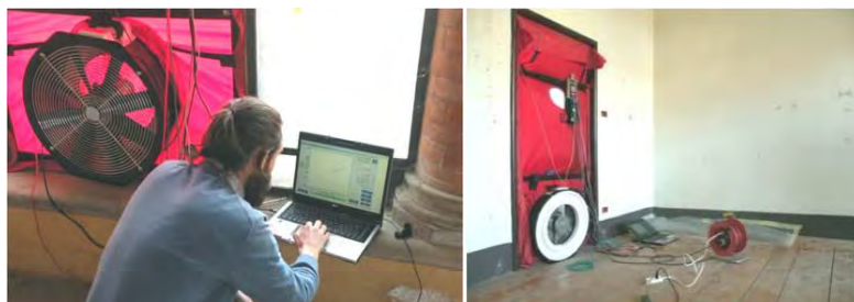
Figure 55_Phases of the blower door test
