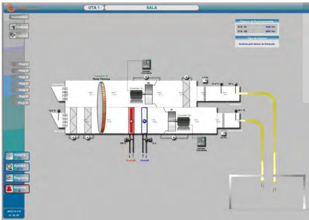
Figure 15_ Interior scheme of RTU
