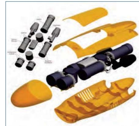
blable parts. The shell's interior gets flooded when the vehicle submerges, hence, floatability is not affected. The external profile has been conceived for hydrodynamic and structural strength and protection of the rotors from direct exposure to objects. The profile has proven its reliability by computational tests of fluid dynamics (CFD).
