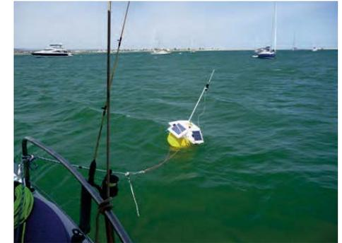
The TP-1 is a telemetry based hydrophone which features a 10/100 MBit/s ethernet interface, which allows direct connection to a computer, or to a wired or wireless network for real-time data streaming to a client that can handle the acoustic data for storage, processing, and/or visualisation. A power/ethernet cable for power supply and two-ways communications can be supplied.
