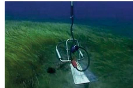
User of XeoTV will get a georeferenced record from a boat during navigation (up to 70 m depth) or stopped (up to 100 m depth). In a single screen the user will get a map of the track, an image window - where the recorded images are shown, plus a text window where the main parameters of the record - name of the file, date, place, company... - and for each frame - GPS coordinates, time... - are displayed.
